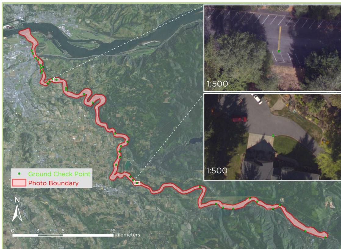
Figure 28: Location of GCPs used to assess the accuracy of the Sandy River orthoimagery
