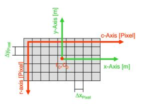
Transformation from Image Coordinate System to Photo Coordinate System
