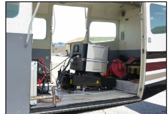
Below: UltraCam Eagle installed in the aircraft.
