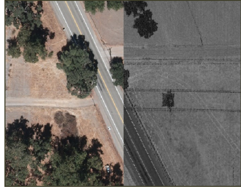
Above: Example of co-registration of color images with LiDAR intensity images. Below: Examples of permanent air targets located within the Lane County project area.
