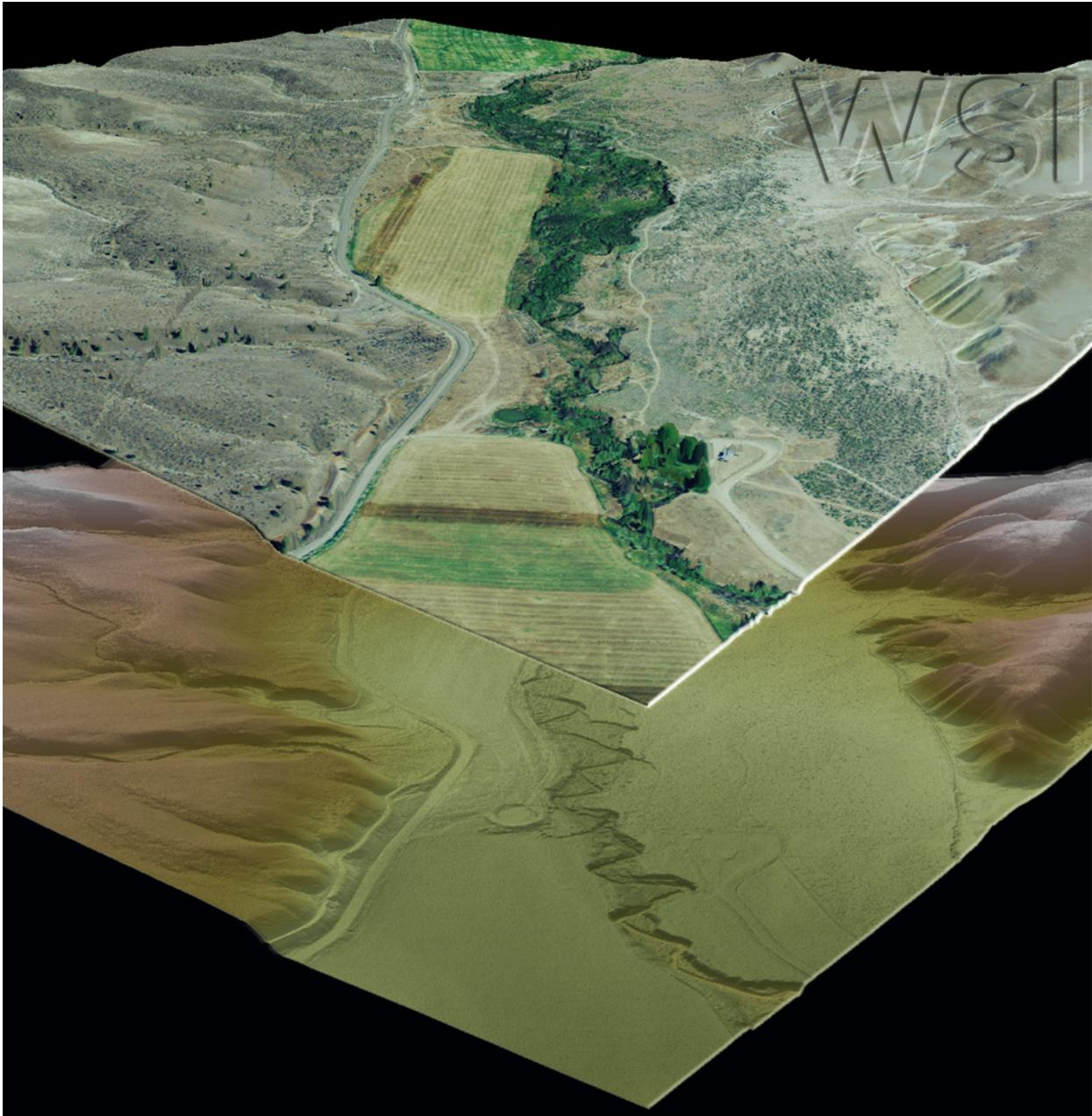
Figure 11: Layered view of the highest hit and bare earth models of a section of Bridge Creek. The top image is the gridded highest hit model colored by 2012 NAIP imagery, the bottom image is the hillshaded bare earth model with all vegetation removed, colored by elevation.
