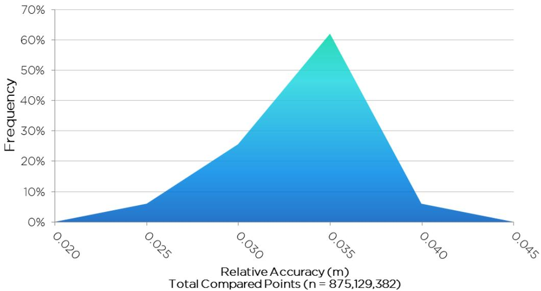
Figure 10: Frequency plot for relative accuracy between flight lines
