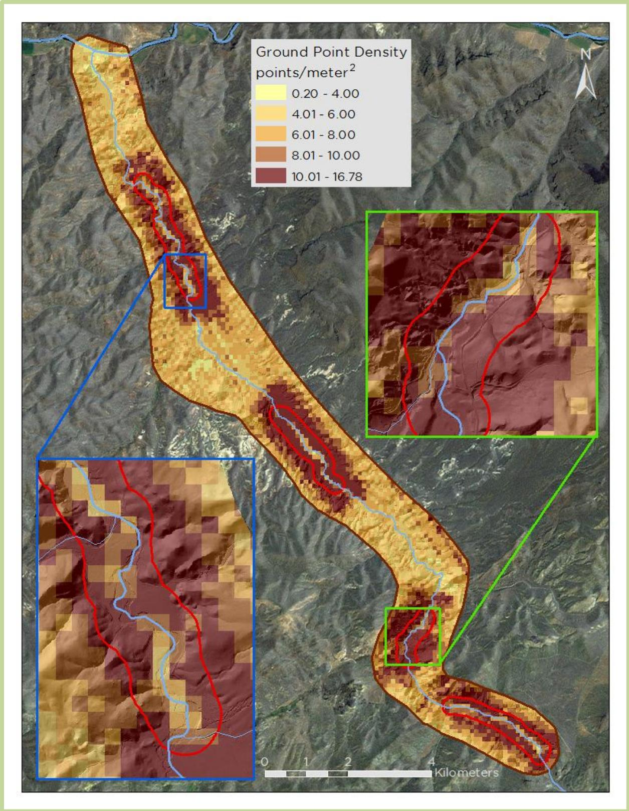
Figure 8: Ground density map for the Bridge Creek LiDAR site
